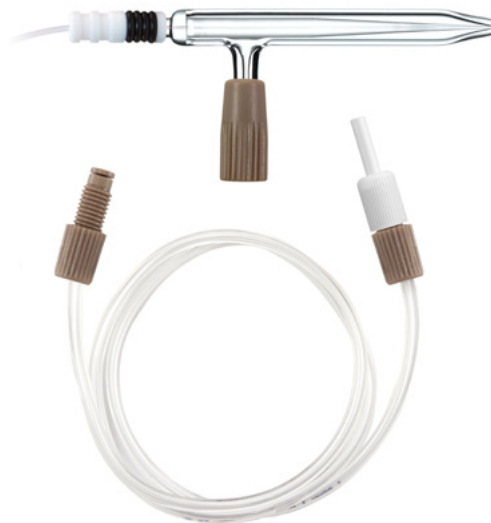
SeaSpray DC Nebulizer for Agilent® 5000 Series GE P/N A13-07-USS2
